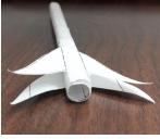
**Step 7:** Bend the fins on each fin unit 90 degrees so that they are each at a right angle to each other. When you look along the back of the rocket, the fins should form a "+" mark.
